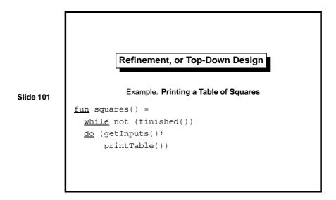
Refinement is top-down design. The main task is expressed as a simple routine that delegates its work to subroutines yet to be defined. You can declare the yet uncoded subroutines as *stubs*: dummy functions that just print their name and exit. (Some systems generate stubs automatically.) With stubs, the program is always executable, even if it doesn't accomplish anything. Coding the lower-level routines adds functionality to the program, so that eventually it can do useful work.
