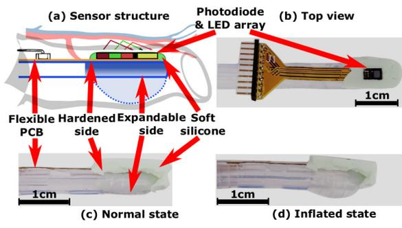
Figure 6: In-ear PPG sensor and balloon design.
