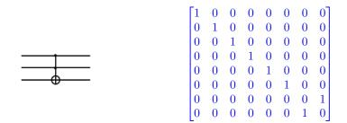
When the first two inputs are classical bits  $(|0\rangle$  or  $|1\rangle$ ), and the third is  $|0\rangle$  the third output is the AND of the first two inputs.
