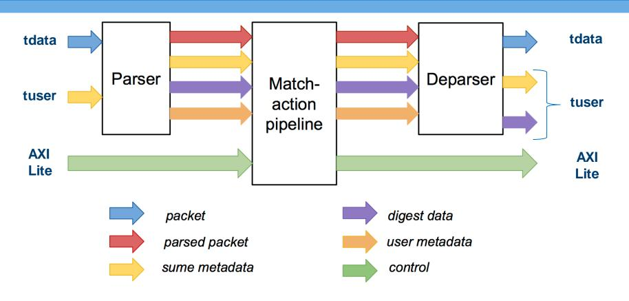
P4 used to describe parser, match-action pipeline, and deparser
