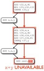
On this path through the flowgraph, x+y is only computed once, so x+y is syntactically unavailable at the last instruction.
