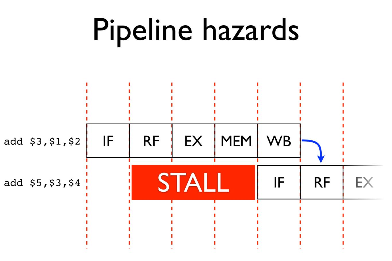
The severity of this effect can be reduced by using bypassing: extra paths are added between functional units, allowing data to be used before it has been written back into registers.
