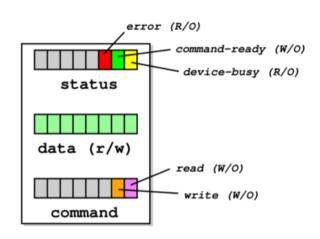
Consider a simple device with three registers: status, data and command. Host can read and write these via bus. Then polled mode operation works as follows:
