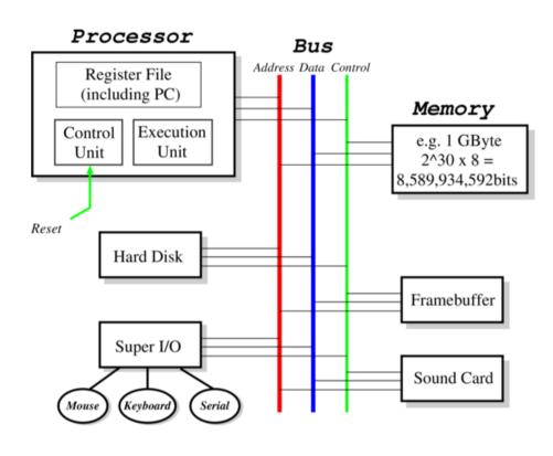
Processor (CPU) executes programs using: **Memory**: stores both programs & data. **Devices**: for input and output. **Bus**: transfers information
