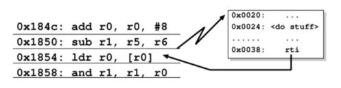
Bus reads and writes are transaction based: CPU requests something and waits until it happens. But, e.g., reading a block of data from a hard-disk might take ~2ms, which could be >5M clock cycles!
