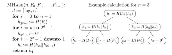
(i) Show that MHASH is not collision resistant if n is not fixed, by constructing two different sequences of files that result in the same output  $h_1$ .
