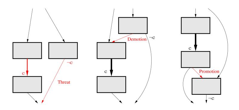
A planner can try to fix a threat by introducing an ordering constraint.
