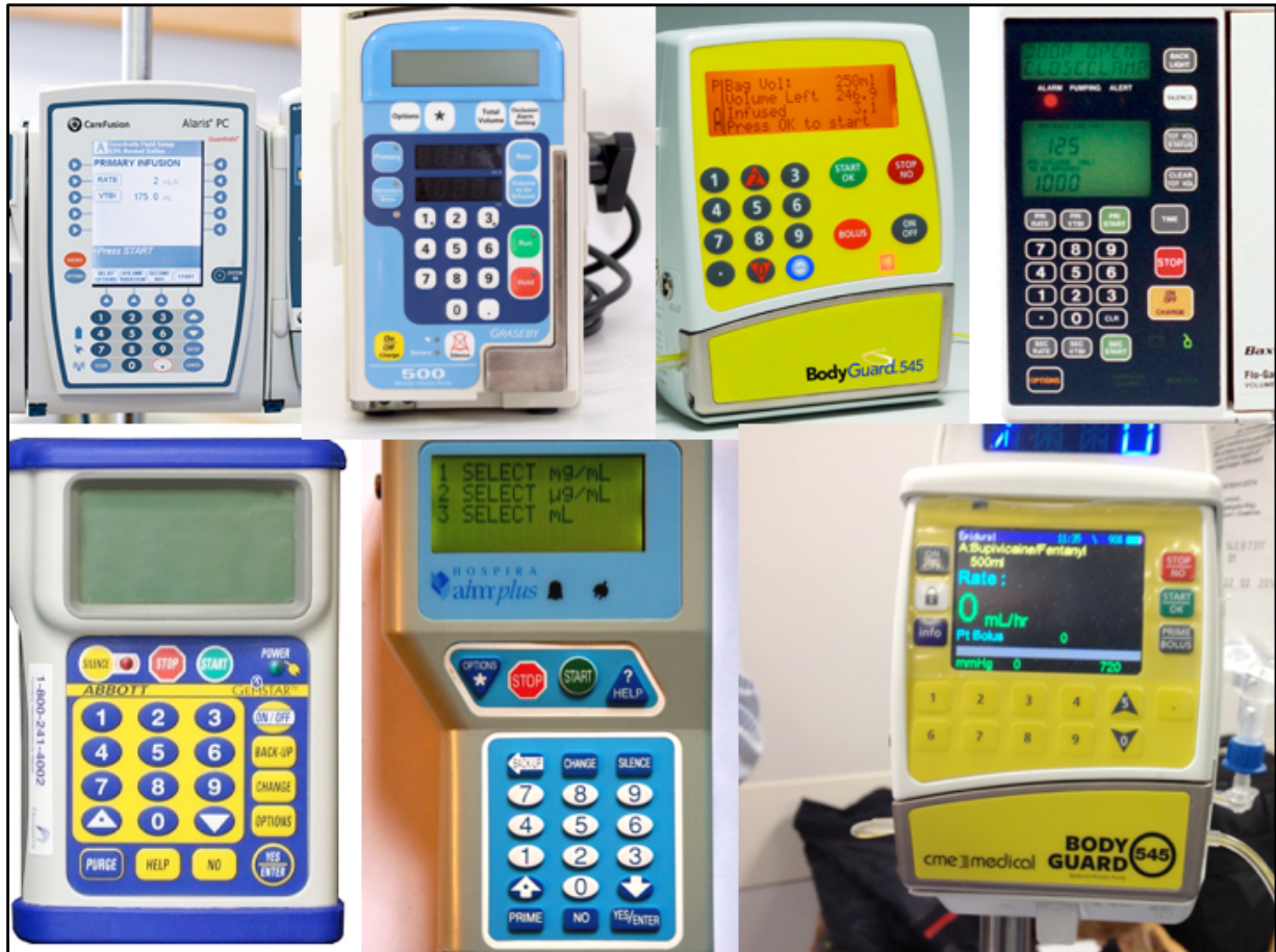
Here are seven infusion pumps. Note that all the controls are different!
