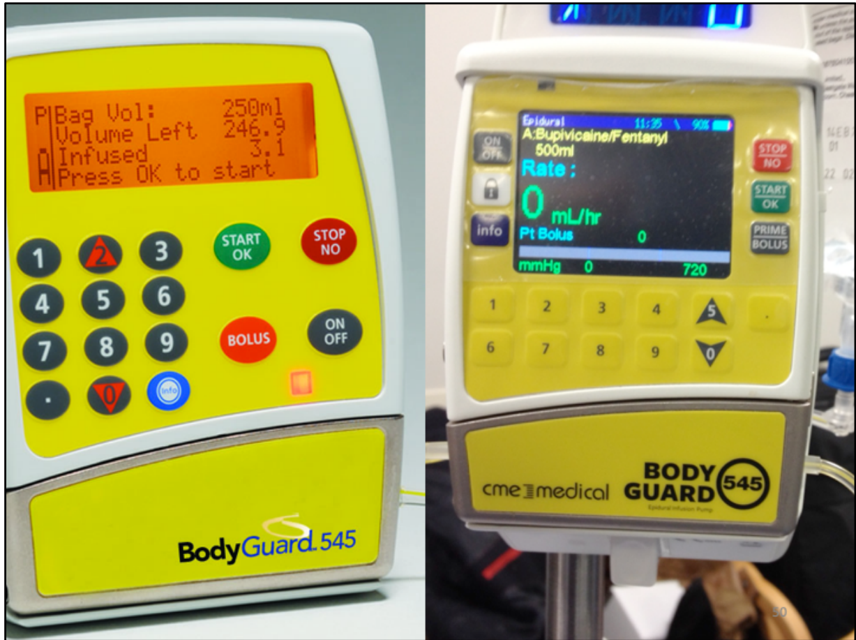
Even the same device make and model (here BodyGuard 545) have different versions with different user interfaces.
