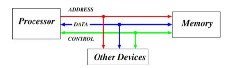
Collection of shared communication wires: low cost, versatile but potential bottleneck. Typically comprises **address lines** (determine how many devices on bus), **data lines** (determine how many bits transferred at once) and **control lines**,
