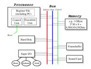
Processor (CPU) executes programs using: Memory: stores both programs & data. Devices: for input and output. Bus: transfers information
