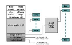
Inside the kernel, a file is represented by a data structure called an index-node or inode which hold file meta-data: owner, permissions, reference count, etc. and location on disk of actual data (file contents)
