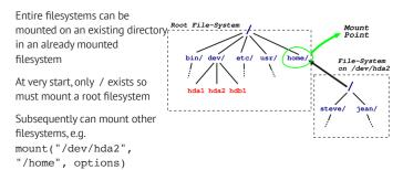
Provides a unified name-space: e.g. access /home/mort/ directly (contrast with Windows9x or NT)
