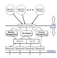
Clear separation between user and kernel portions was the big difference between Unix and contemporary systems – only the **essential** features *inside* OS, not the editors, command interpreters, compilers, etc.
