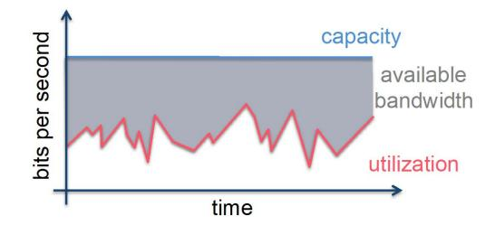
End-to-end capacity and End-to-end effective bandwidth
