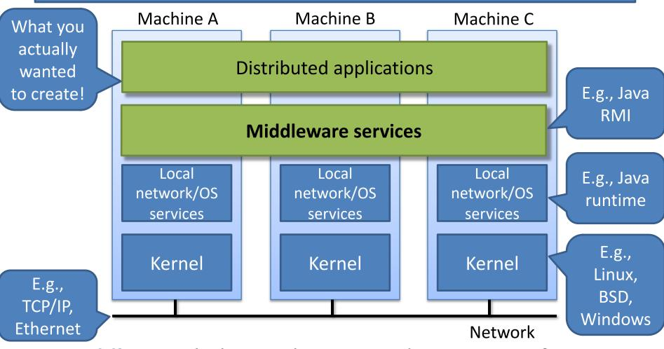
• **Middleware** helps application authors write software intended to run on more than one machine at a time.
