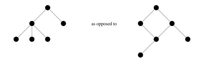
In a *tree* only *one path* can lead to a given state. In a *graph* a *state* can be reached via possibly *multiple paths*.
