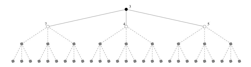
Initially, the algorithm looks ahead and finds the *smallest* f cost that is *greater than* its current f cost limit. The new limit is 4.
