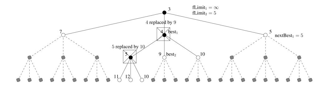
Now  $f(\text{best}_2) > \text{fLimit}_2$  so the function call returns (fail, 9) into (result<sub>2</sub>, f') and  $f(\text{best}_1) = 9$ .
