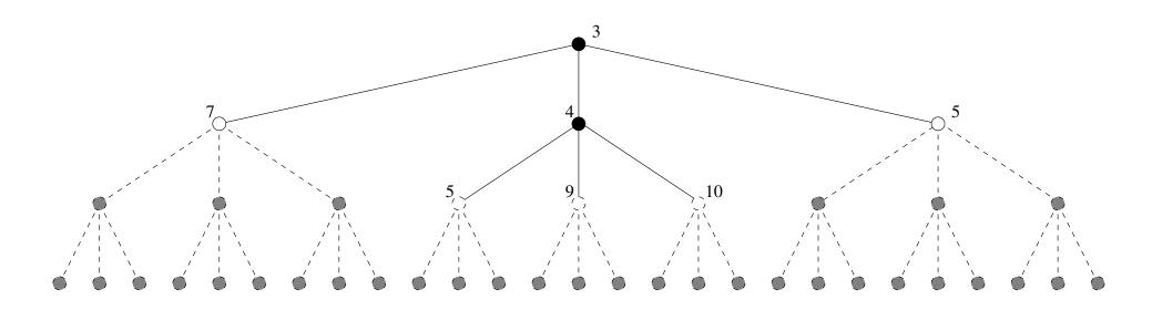
Anything with f cost *at most* equal to the current limit gets explored, and the algorithm keeps track of the *smallest* f cost that is *greater than* its current limit. The new limit is 5.
