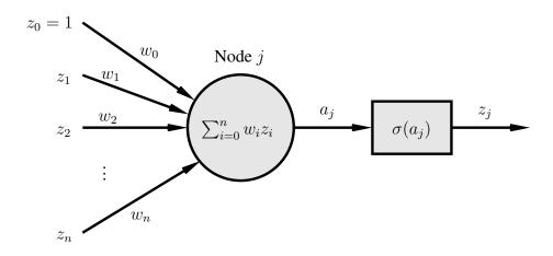
Weights  $w_i$  connect nodes together, and  $a_j$  is the weighted sum or activation for node j.  $\sigma$  is the activation function and the output is  $z_j = \sigma(a_j)$ .
