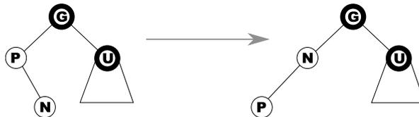
When in **case 2** ( $n, p$  red,  $g, u$  black,  $g \rightarrow p \rightarrow n$  is a zig-zag, as above), perform a rotation on the  $p - n$  edge to transform the zig-zag into a straight  $g \rightarrow n \rightarrow p$ . Note how this has made  $n$  the parent of  $p$ , so the names are no longer appropriate. If you swap the names of  $n$  and  $p$ , however, you are now in case 3.
