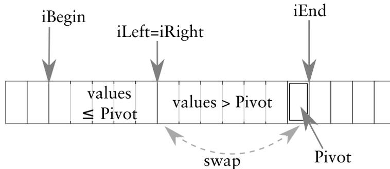
At that point, when  $iLeft = iRight$ , we put the pivot in its rightful place between the two regions we created, by swapping  $A[iRight]$  and  $A[iEnd - 1]$ .
