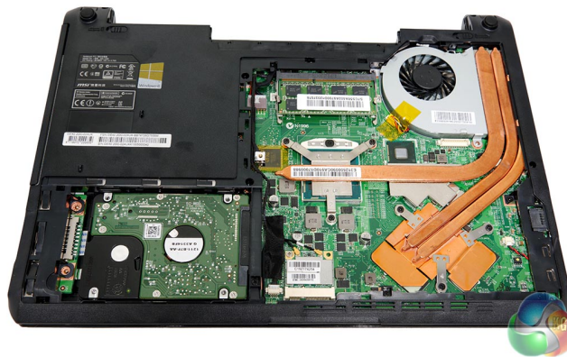
Figure 1.16: Thermal management heat pipes in a modern laptop.
