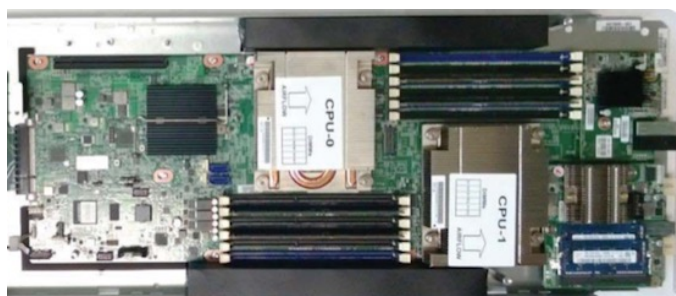
Figure 3.5: Catapult Blade - FPGA is at the lower right, its heatsink visible above its blue DRAM DIMMs.
