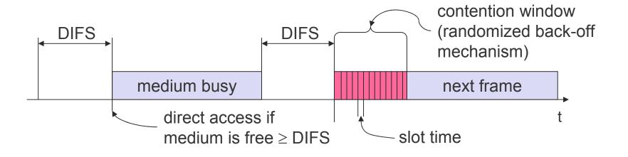
CSMA/CA: sense medium. If free transmit (although this might generate collision at the receiver). If not, wait with a back off strategy. Transmit when medium is sensed free.
