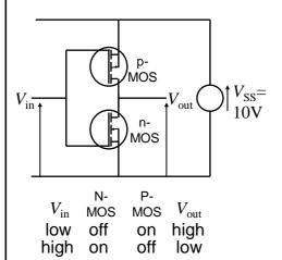
Using the graphical approach we can show that the switching characteristics are now much better than for the n-MOS inverter
