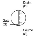
The current flow from D to S  $(I_{\rm DS})$  is controlled by the voltage applied between G and S  $(V_{\rm GS})$
