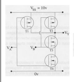
$V_A$   $V_B$  T1 T2 T3 T4  $V_Y$  low low on on off off high low high on off on off high high low off on off on high high high off off on on low
