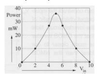
This is when both transistors are on. When one or the other is off, the power dissipation is zero
