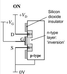
Consider the situation when the Gate (G) voltage ( $V_{\rm G}$ ) is raised to a positive voltage, say  $V_{\rm D}$
