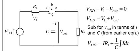
$$V_{DD} - V_1 - V_{out} = 0$$
