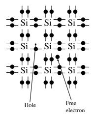
As temperature rises, thermal vibration of the atoms causes bonds to break: electrons are free to wander around the crystal.
