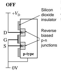
Drain (and Source) diode reverse biased, so no path for current to flow from S to D, i.e., the transistor is **off**
