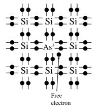
The additional electron needs only a little energy to move into the conduction band.
