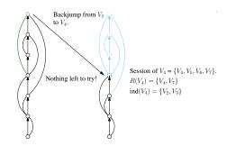
As expected, we back jump to  $V_3$  instead of  $V_2$ . Hooray!
