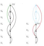
Backjumping from  $V_7$  to  $V_4$  is fine. However we shouldn't then just backjump to  $V_2$ , because changing  $V_3$  could fix the problem at  $V_7$ .
