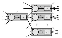
Because we know how to compute  $\delta_j$  for the output node we can work backwards computing further  $\delta$  values.
