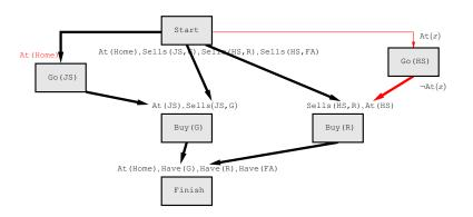
The  $At({\tt HS})$  precondition is easy to achieve. But if we introduce a causal link from Start to  $Go({\tt HS})$  then we risk invalidating the precondition for  $Go({\tt JS})$ .
