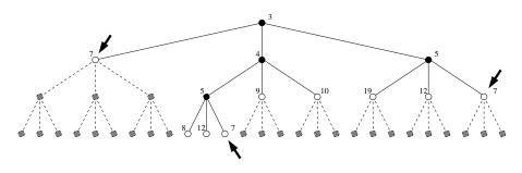
The new limit is 7, so at the next iteration the three arrowed nodes will be explored.
