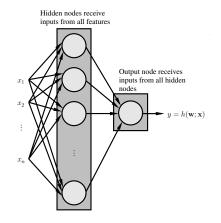
For the output:  $\sigma(a) = a$ . For the hidden nodes  $\sigma(a) = \frac{1}{1 + \exp(-a)}$ .
