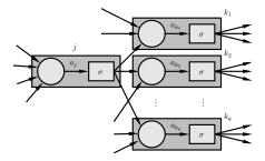
$$\frac{\partial a_k}{\partial a_j} = \frac{\partial}{\partial a_j} \left( \sum_i w_{i \to k} \sigma(a_i) \right) = w_{j \to k} \sigma'(a_j)$$
