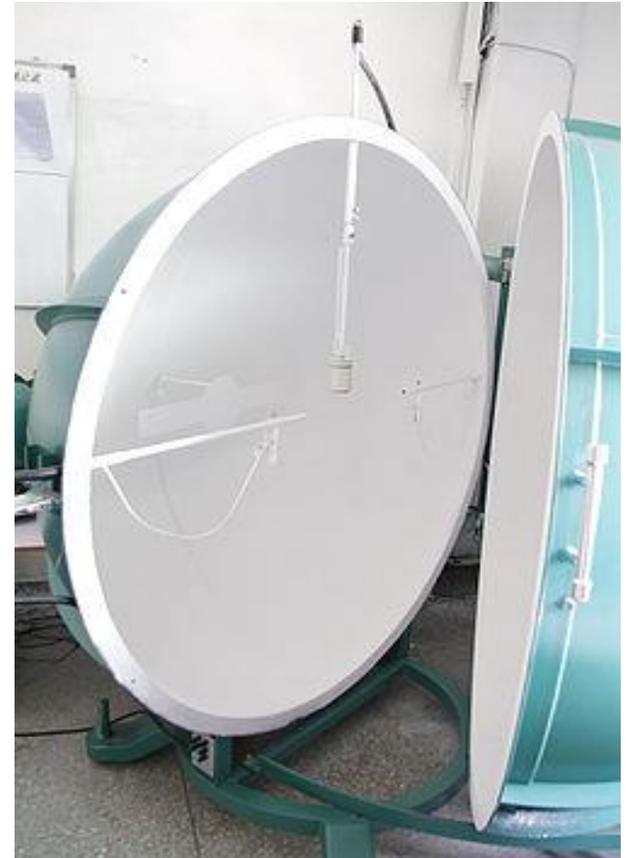
Integrating sphere – to measure all light emitted
