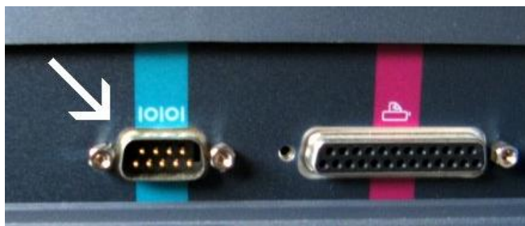
Figure 1.10: Typical Serial and Parallel Ports of 20th Century
