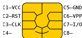
Figure 1.7: Contact plate for a smartcard - Reader supplies VCC power, clock and reset. I/O is via the one-bit, bidirectional data pin .
