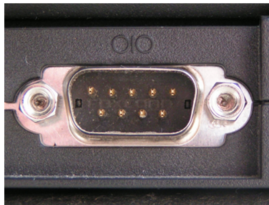
Figure 1.12: Serial Port Connector (9 pin instead of original 25 pin).
