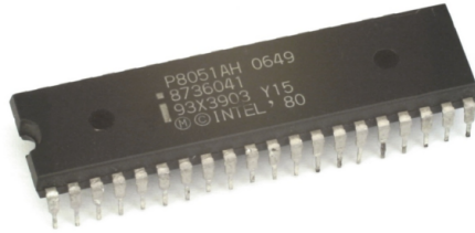
Figure 1.5: Intel 80C51 Microcontroller Chip from 1980.
