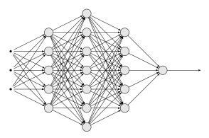
Here, each *node* is a perceptron and each *edge* has a weight attached.
