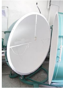
Integrating sphere – to measure all light emitted
