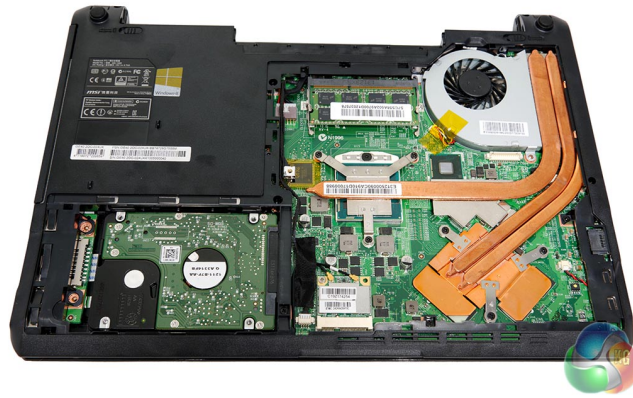
Figure 2.10: Thermal management heat pipes in a modern laptop.
