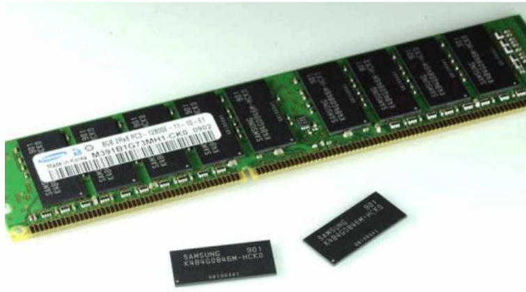
Figure 1.28: DRAM single-in-line memory module (SIMM).
