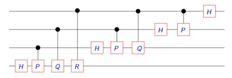
In the input, the least significant bit is at the top, in the output, it is at the bottom.
