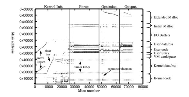
In a short time interval, the locations referenced by a process tend to be grouped into a few regions in its address space:
