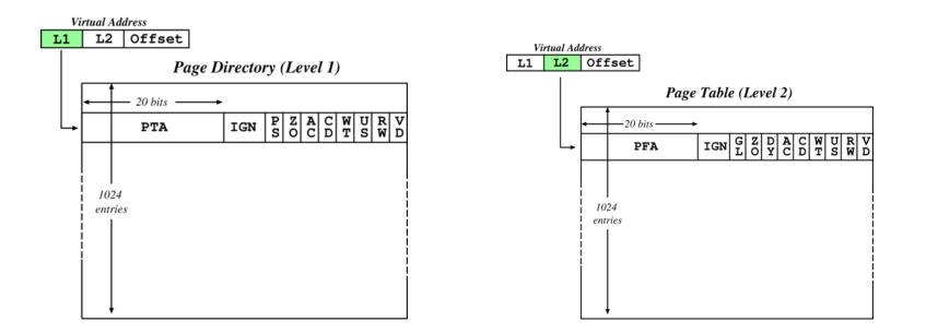
Page size is 4kB or 4MB. First lookup to the **page directory**, indexed using top 10 bits. The page directory address is stored in an internal processor register (cr3). The lookup results (usually) in the address of a page table. Next 10 bits index the **page table**, retrieving the **page frame address**. Finally, add in the low 12 bits as the **page offset**. Note that the page directory and page tables are exactly one page each themselves (not by accident)
