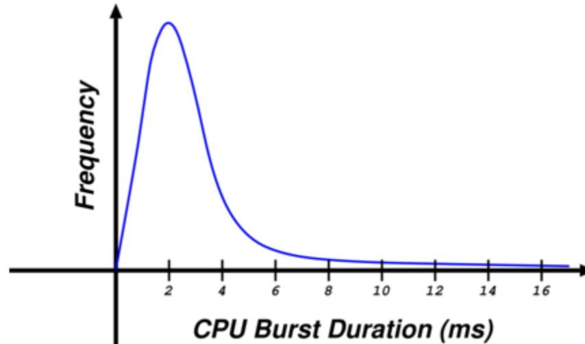
Observe that most processes execute for at most a few milliseconds before blocking
