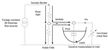
This drawing may suggest the water from the channel spills into the pool. But such an arrangement would be like the Kubla Falls and the flow rate would be unaffected by the current depth. In reality the channel joins the pool below the waterline, and hence backpressure applies.
