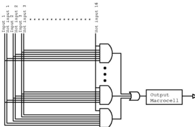
The output from the each OR gate is connect to an output pin through an output macrocell. This can be programmed to latch (using a D-type FF) the output or feed the output signal back into AND array. For a more detailed description of this PAL, read the datasheet.
