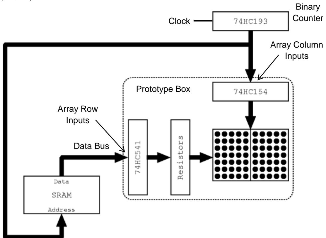
The array should now display the random contents (since we have not written any specific data to the SRAM yet) held in the SRAM. Turn your power supply on and off several times to see if the pattern changes on the LED arrays. Make sure you leave the circuit turned-off for at least 20s!
