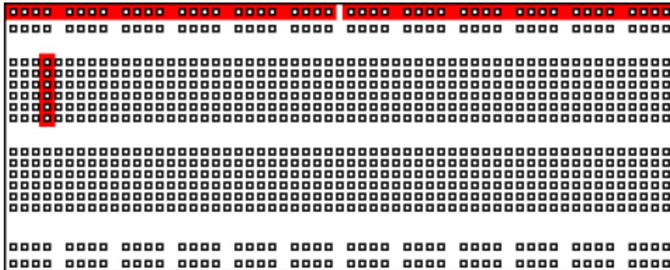
These strips connect the holes on the top of the board. This makes it easy to connect components together to build circuits. To use the breadboard, the legs of components are placed in the holes (the sockets). The holes are made so that they will hold the component in place. Each hole is connected to one of the metal strips running underneath the board.
