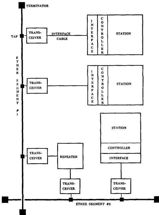
the intended receivers. The Ether is a logically passive medium for the propagation of digital signals and can be constructed using any number of media including coaxial cables, twisted pairs, and optical fibers.
