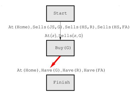
Thick arrows denote causal links. They always have a thin arrow underneath. Here the new Buy step achieves the Have(G) precondition of Finish. The planner can now introduce a second causal link from Start to achieve the Sells(x, G) precondition of Buy(G).
