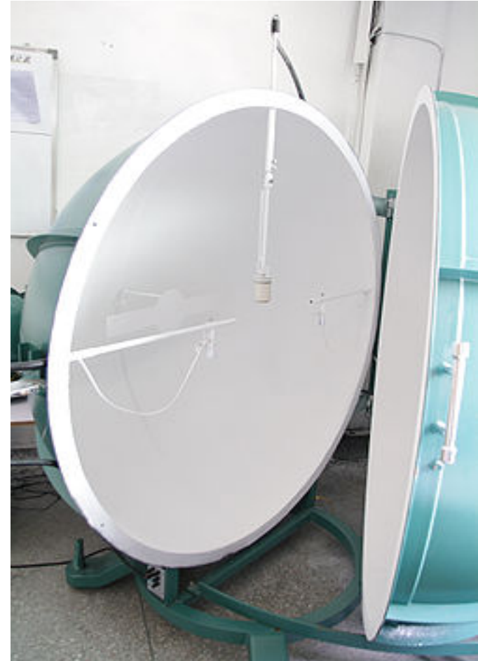
Integrating sphere – to measure all light emitted
