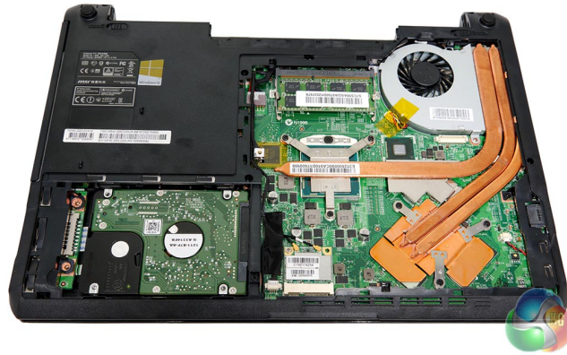
Figure 2.8: Thermal management heat pipes in a modern laptop.
