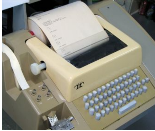
Figure 1.12: Teletype/teleprinter: These devices were almost entirely mechanical with the electric circuit being little more than one switch activated by cams for transmit and one solenoid for receive.
