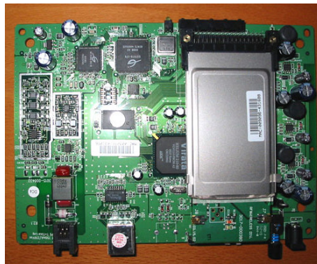
Figure 1.32: Helium chip as part of a home gateway ADSL modem (partially masked by 802.11 module).
