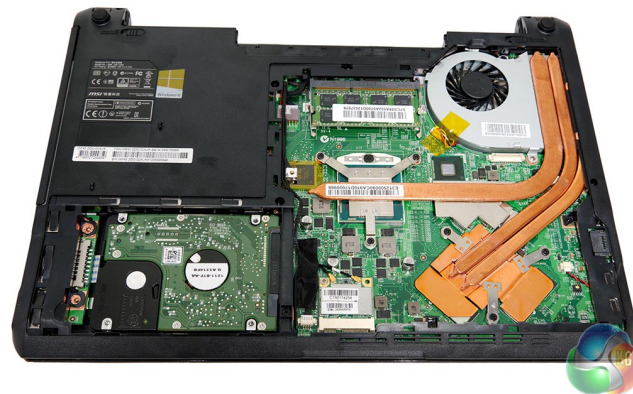
Figure 2.9: Thermal management heat pipes in a modern laptop.
