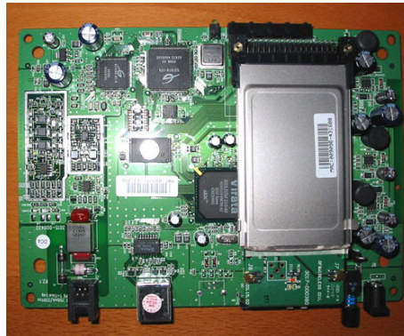
Figure 1.23: Helium chip as part of a home gateway ADSL modem (partially masked by 802.11 module).
