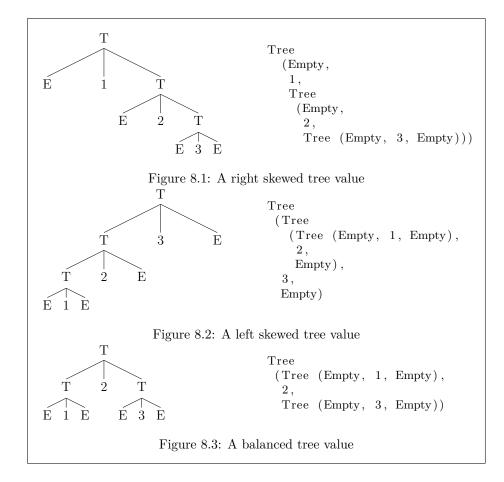
Using the constructors of tree we can build a variety of tree values. For example, we can build trees that are skewed to the right (Figure 8.1) or to the left (Figure 8.2), or whose elements are distributed evenly between left and right (Figure 8.3).
