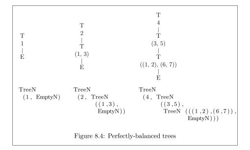
the elements are distributed evenly to the left and to the right. As a result, the only trees that can be built are perfectly balanced trees whose elements number one less than a power of two (Figure 8.4).
