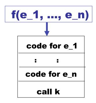
This will leave the values of each arg on the stack, with the value of e\_n at the top. Here k is the address for the start of the code for f.
