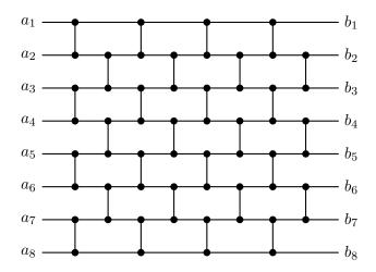
As can be seen in the figure, for  $i=1,2,\ldots,n$  and  $d=1,2,\ldots,n$ , line i is connected by a depth-d comparator to line  $j=i+(-1)^{i+d}$  if  $1\leq j\leq n$ .
