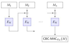
Similar to CBC:  $IV = 0^m$ , last ciphertext block serves as tag. Provides existential unforgeability, but only for **fixed** message length n: Adversary asks oracle for  $T^1 := \text{CBC-MAC}_{E_K}(M^1) = E_K(M^1)$  and then presents  $M = M^1 || (T^1 \oplus M^1)$  and  $T := \text{CBC-MAC}_{E_K}(M) = E_K((M^1 \oplus T^1) \oplus E_K(M^1)) = E_K((M^1 \oplus T^1) \oplus T^1) = E_K(M^1) = T^1$ .
