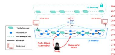
Figure 1: A SCION L3.5 overlay on top of an IP L3 loses its security benefits.
