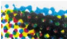
150 lpi  $\times$  16 dots per cell = 2400 dpi phototypesetter (16 $\times$ 16 dots per cell = 256 intensity levels)
