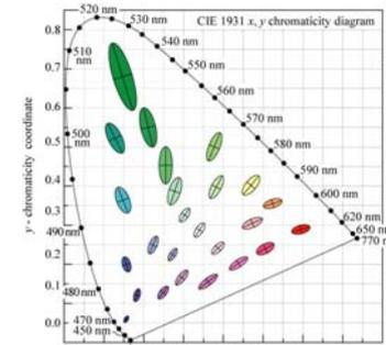
Fig. 17.5. MacAdam ellipses plotted in the CIE 1931  $(x, y)$  chromaticity diagram. The axes of the ellipses are ten times their actual lengths (after MacAdam, 1943; Wright, 1943; MacAdam, 1993).
