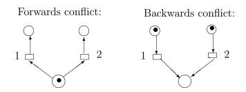
Either one of events 1 and 2 can occur, but not both. This shows how nondeterminism can be represented in a basic net.
