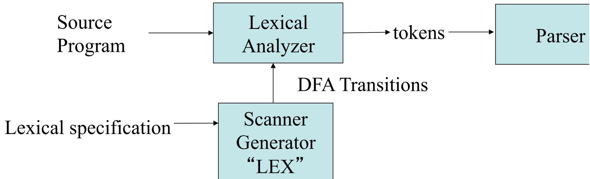
The idea : use regular expressions as the basis of a lexical specification. The core of the lexical analyzer is then a deterministic finite automata (DFA)
