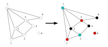
Each node corresponds to a *variable*. We have three colours and directly connected nodes should have different colours.
