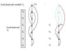
Given an instantiation  $I_k$  and  $V_{k+1}$ , if there is no consistent  $d \in D_{k+1}$  we call  $I_k$  a *leaf dead-end* and  $V_{k+1}$  a *leaf dead-end variable*.
