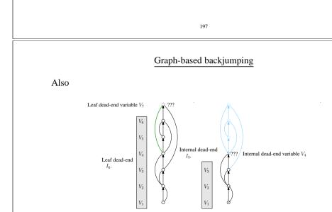
If  $V_i$  was backtracked to from a later leaf dead-end and there are no more values to try for  $V_i$  then we refer to it as an *internal dead-end variable* and call  $I_{i-1}$  an *internal dead-end*.
