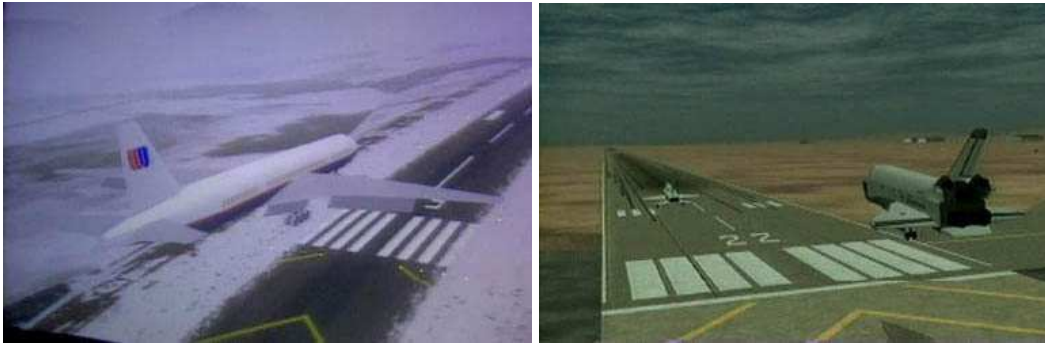
Figure 6: Screen shots from commercial flight simulators, circa 1995. The graphics used today are better than this, but not as good as you see in video games: most aircraft cockpits are a long way away from the scenery for most of the time, and pilots spend most of their time looking at the instruments, rather than looking out the window.
