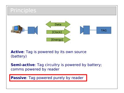
The broad definition of RFID means that there has to be a lot of flexibility in what is supported. So the reader might supply a clock signal, or not.
