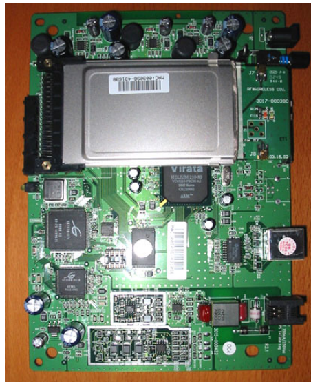
Figure 7.19: Helium chip as part of a home gateway ADSL modem (partially masked by 802.11 module).
