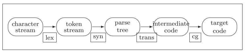
A *multi-pass compiler* does one 'simple' thing at once and passes its output to the next stage.
