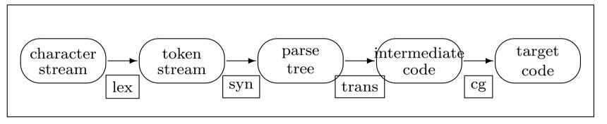
Type checking often not mentioned explicitly. Here you can think of it as being an arrow from *parse tree* to *parse tree* which checks types (rejecting ill-typed programs) and fixes up the parse tree.
