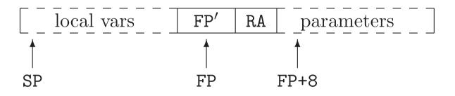
Space below (to the left of) the stack frame is used to construct the argument list (possibly empty) of any called routines—the called routine then turns this into a 'proper' stack frame.
