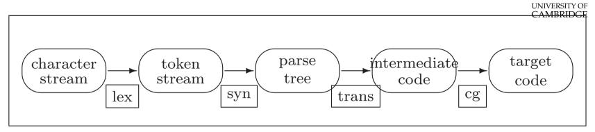
A classical compiler does all these on one machine. To distribute a system for multiple architectures we compile it once per architecture. When running Java in a Browser, the JVM file is transported after the first 3 stages of compilation. The recipient browser may:
